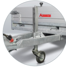
Long drawbar with automatic jockey wheel
