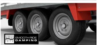
• Smooth-ride, self damping T Transporters are all designed for long distance and heavy loads. Axles and suspension technology is by AL-KO, Europe's largest trailer equipment manufacturer.
